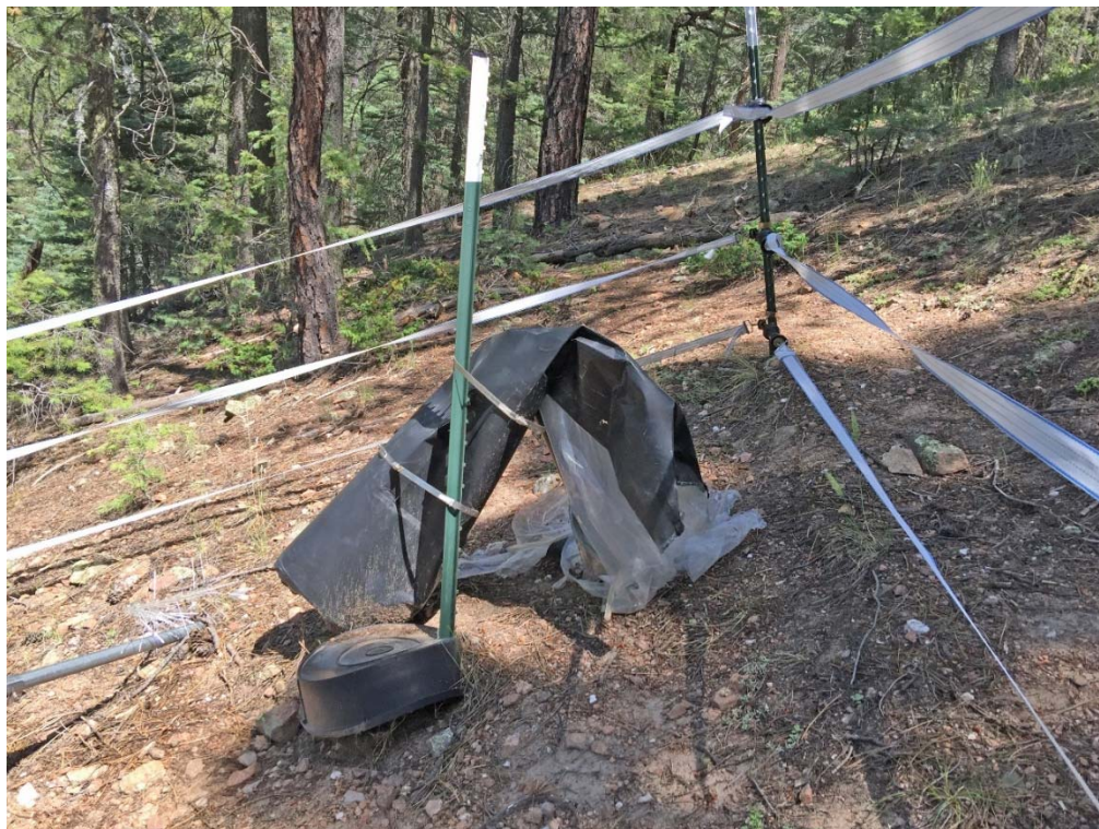
Figure 5. Bear Damage to Lower Precipitation Station observed July 2019.
