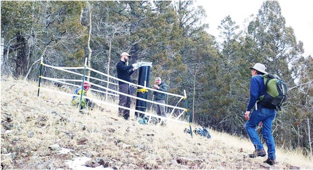
Figure 4. Installation of the Upper 2 precipitation collector.
